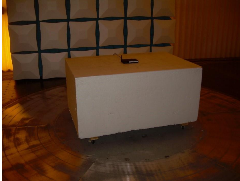
Photograph 1: Front View Radiated Emissions Below 1000 MHz Configuration
