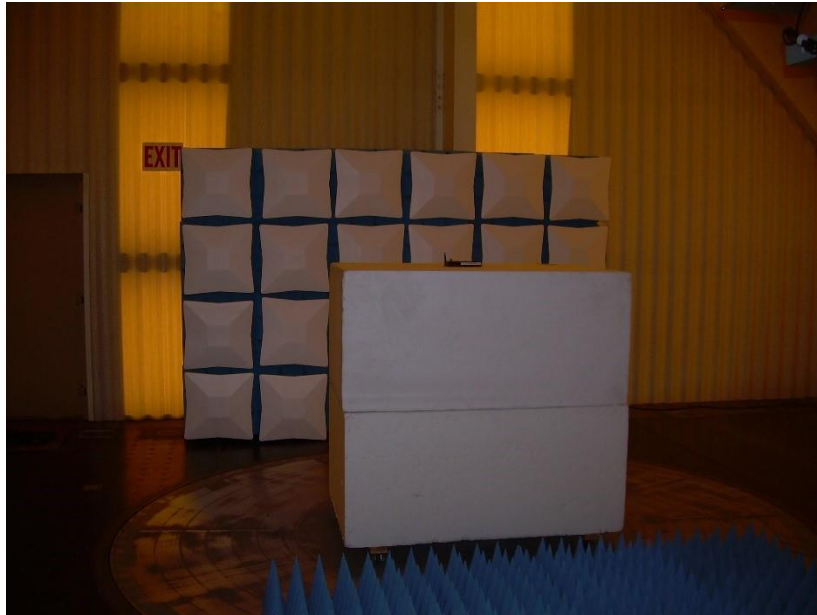
Photograph 3: Front View Radiated Emissions Above 1000 MHz Configuration
