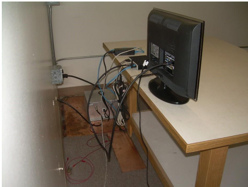
Photograph 6: Back View Conducted Emissions Worst-Case Configuration
