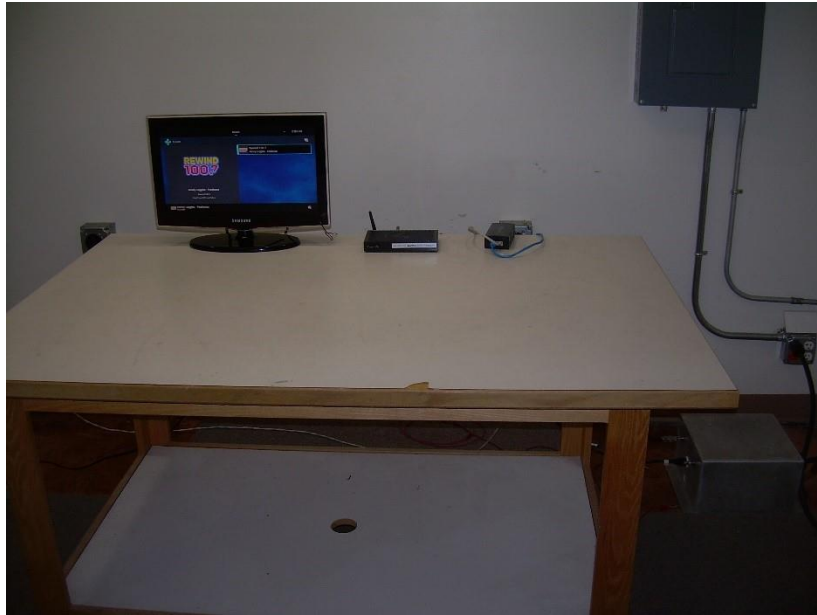
Photograph 5: Front View Conducted Emissions Worst-Case Configuration
