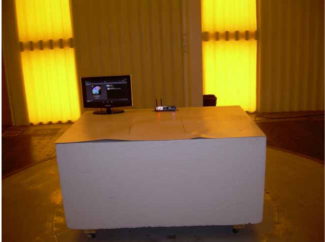
Photograph 1 – Front View Radiated Disturbance Configuration – Oxford TEC Antenna
