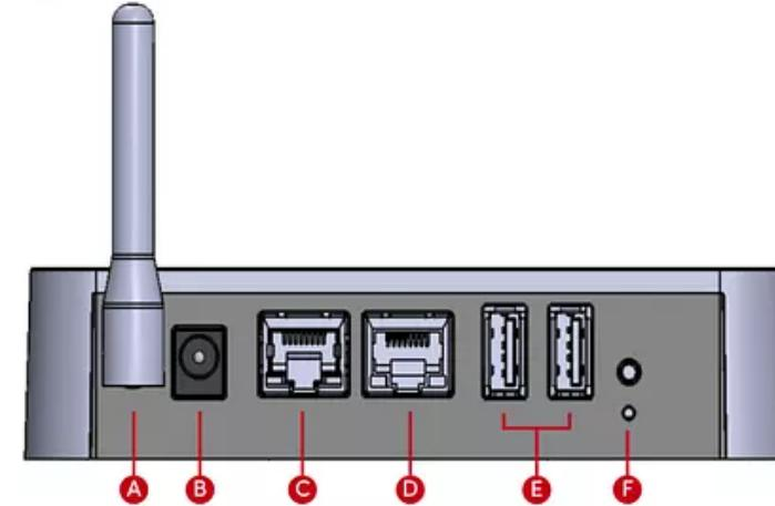
**A** **Zigbee**—External antenna connector for Zigbee radio.
