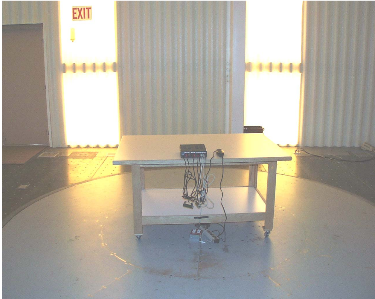
Photograph 2 - Back View Radiated Disturbance Worst Case Configuration
