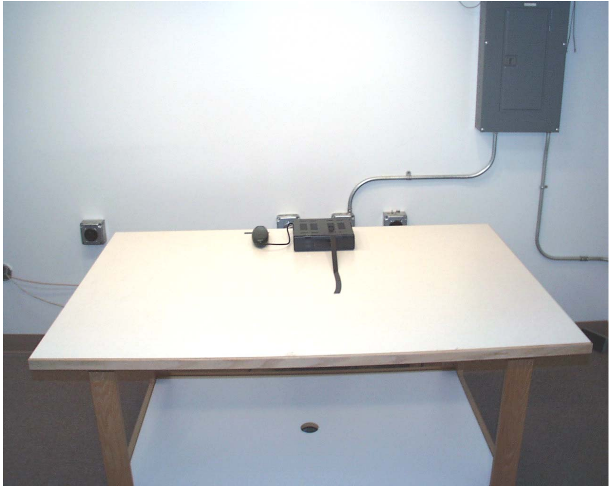
Photograph 3 - Front View Conducted Disturbance Worst Case Configuration
