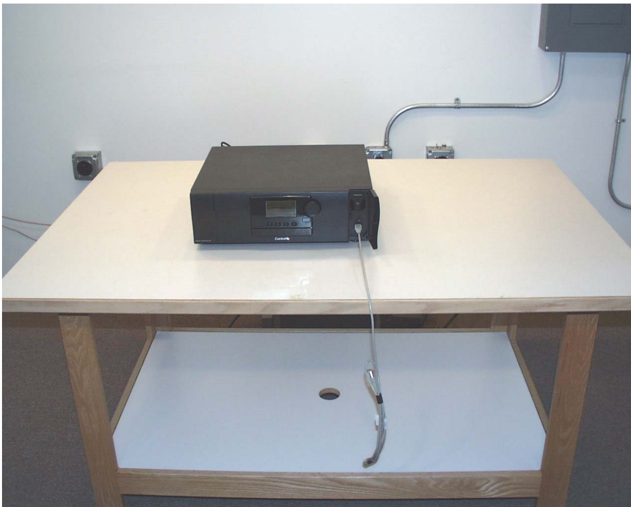
Front View Conducted Disturbance Worst Case Configuration
