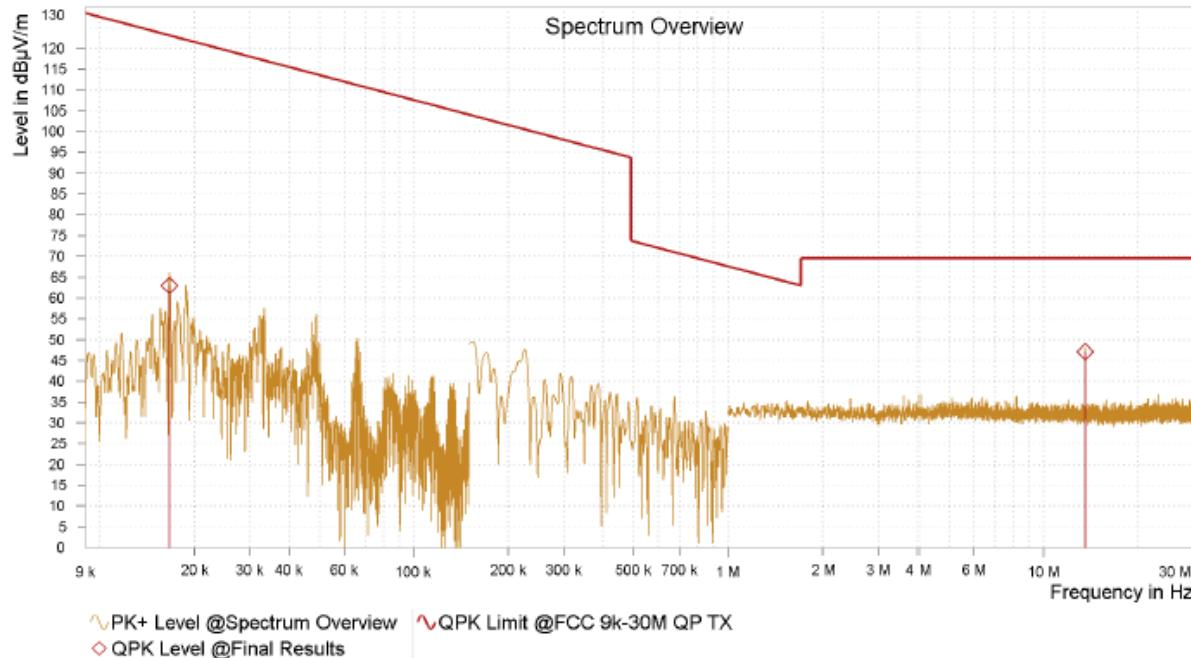
**Radiated Spurious Emission 30 MHz – 1 GHz : HF ASK**
