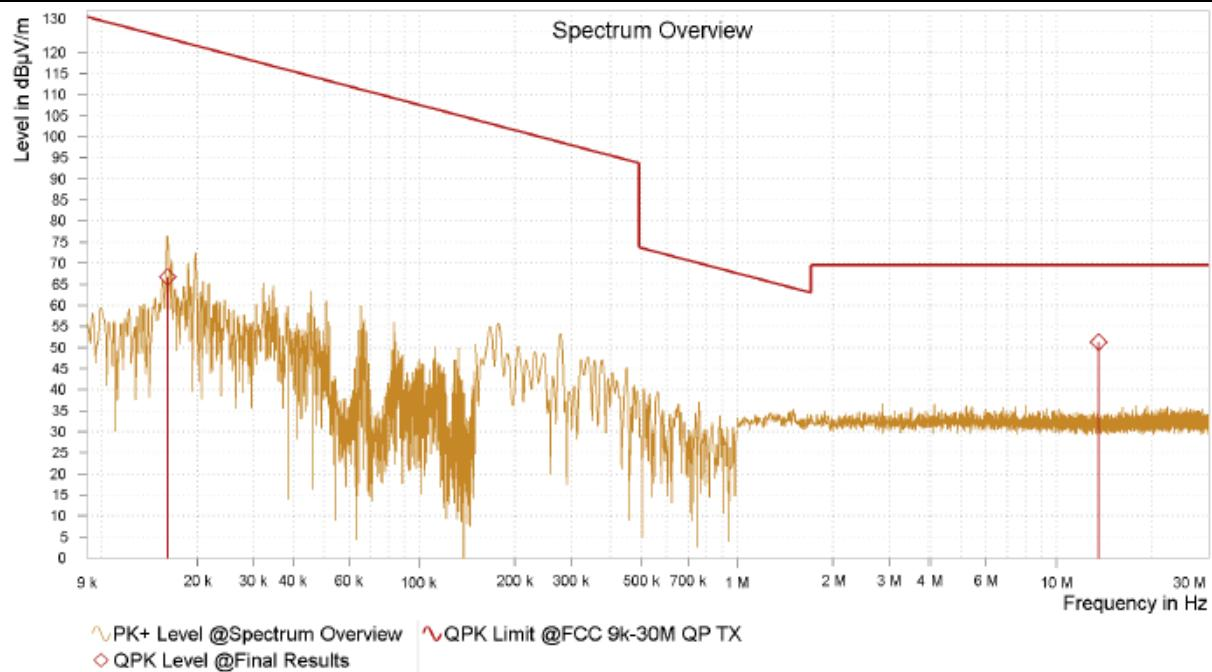
**Radiated Spurious Emission 9 kHz – 30 MHz (Antenna Position 180°) : HF ASK**
