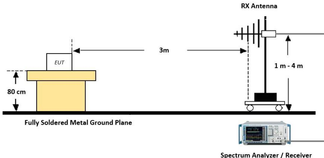
**Test Procedure of Radiated spurious emissions (Below 1GHz)**
