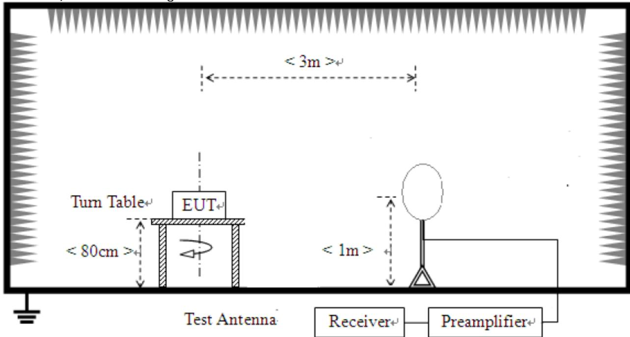
2) For field strength of emissions from 30 MHz to 1 GHz
