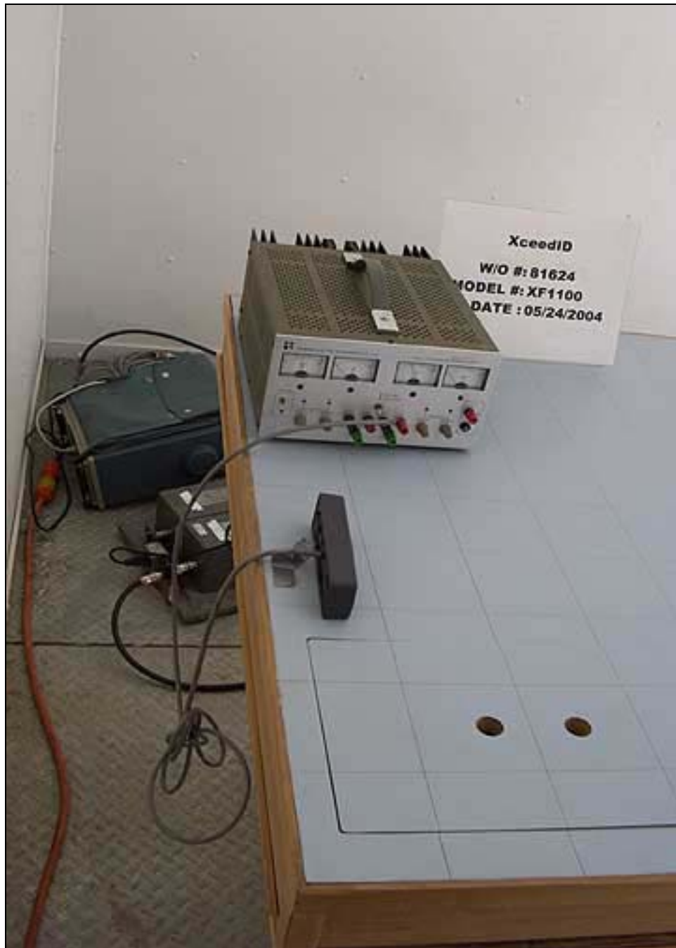
Mains Conducted Emissions - Side View
