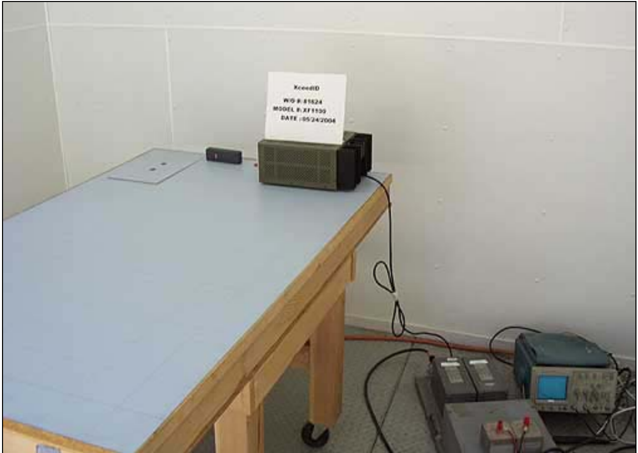
Mains Conducted Emissions - Front View
