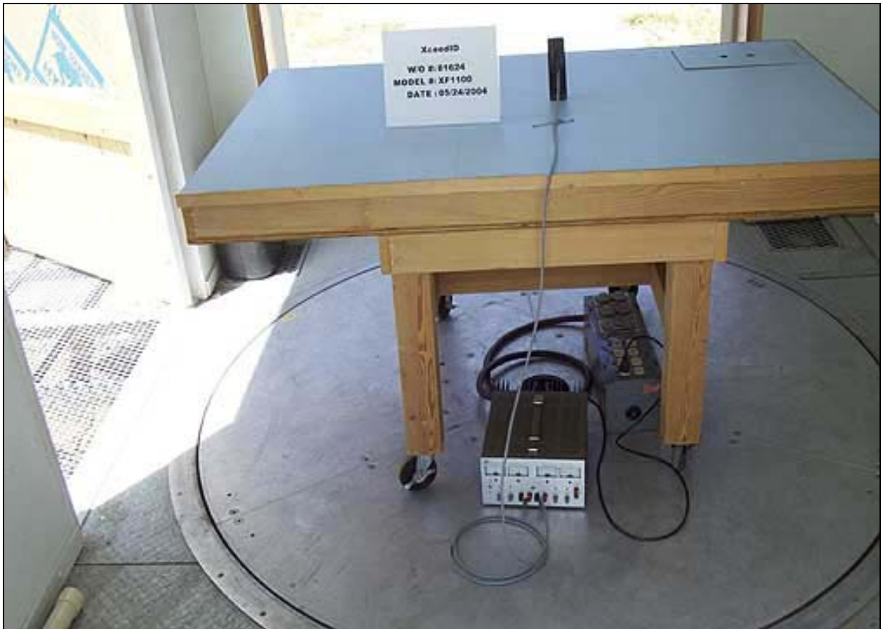
Radiated Emissions - Back View
