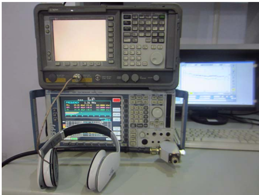
SPURIOUS EMISSION TEST SETUP
