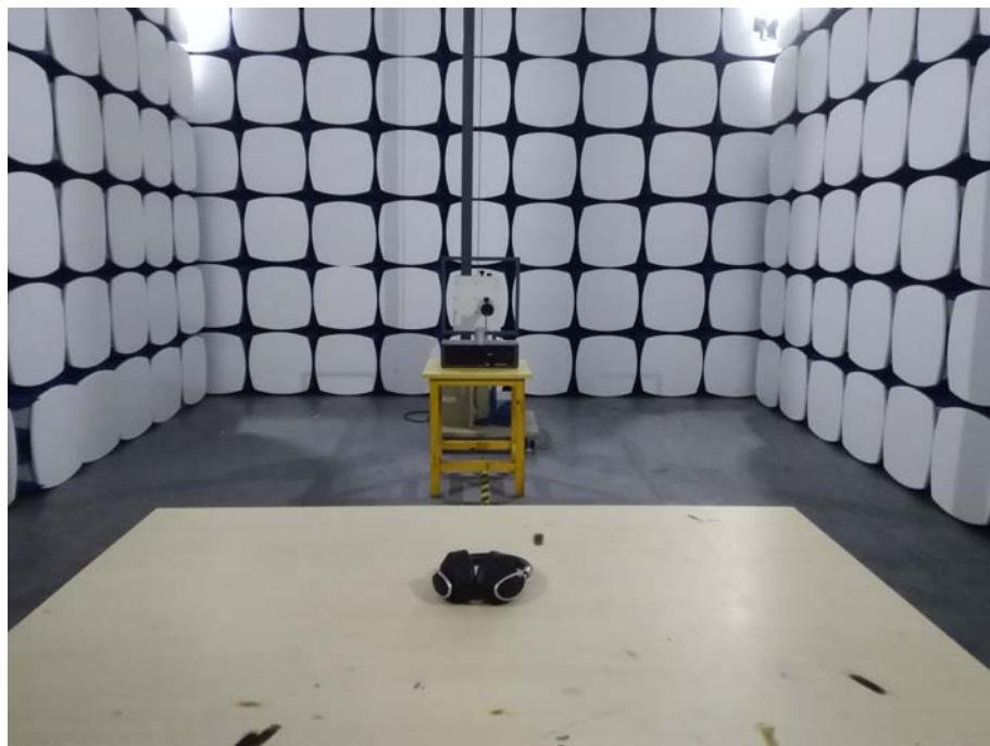
**Radiation Emission Test Setup (30MHz to 1GHz)**
