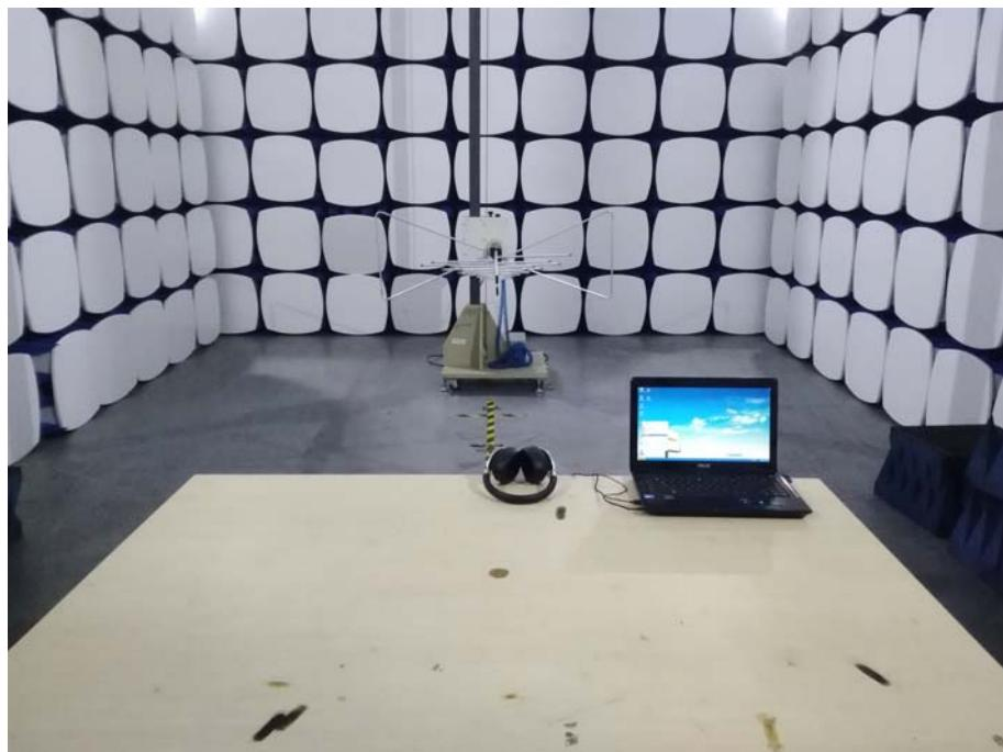
**Radiation Emission Test Setup (Above 1GHz)**
