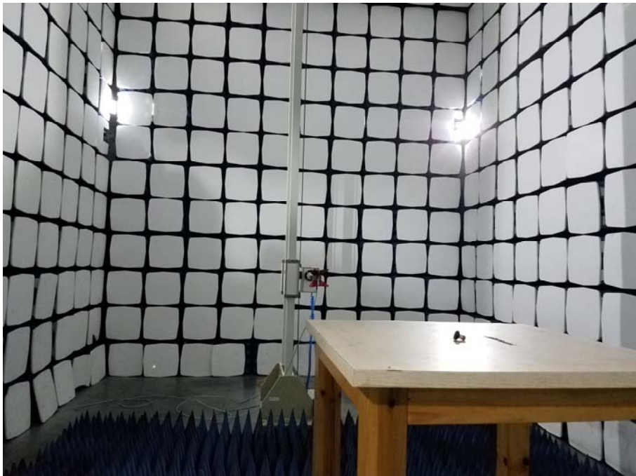
Radiation Emission Test Setup (Above 1GHz)
