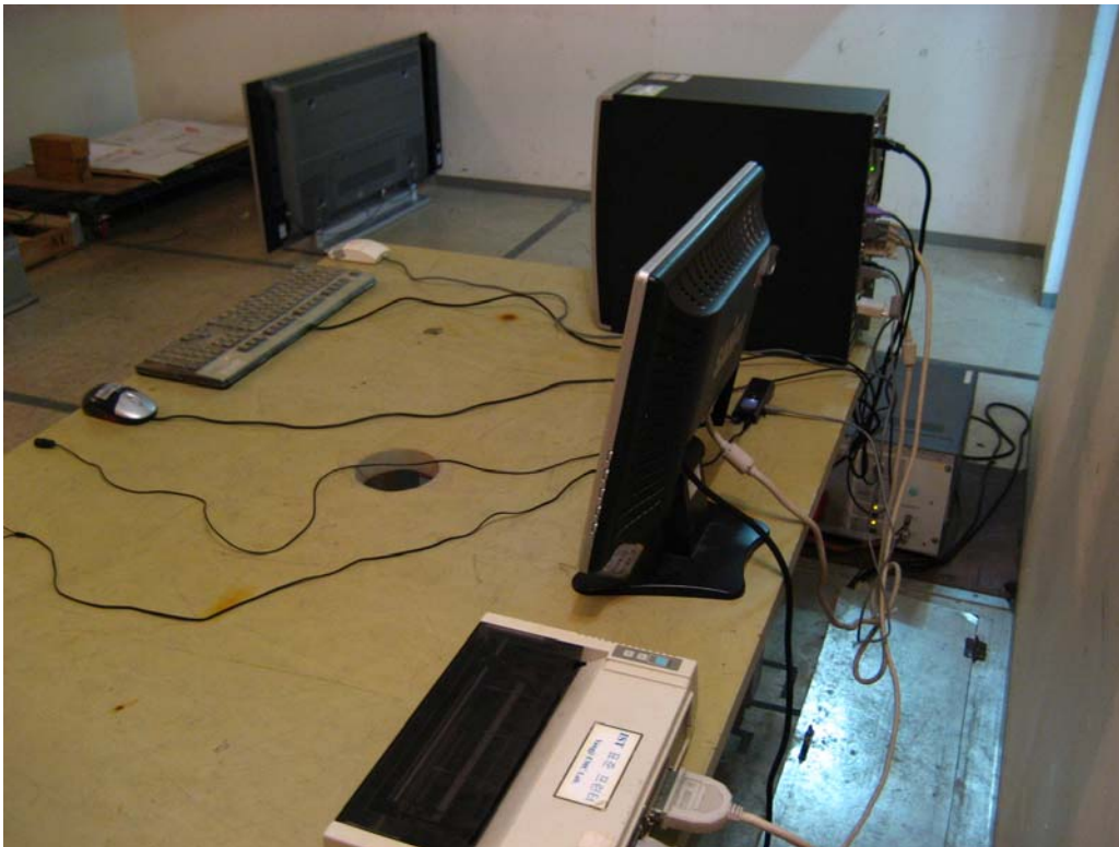
Conducted Emissions (PC power line) - Rear View
