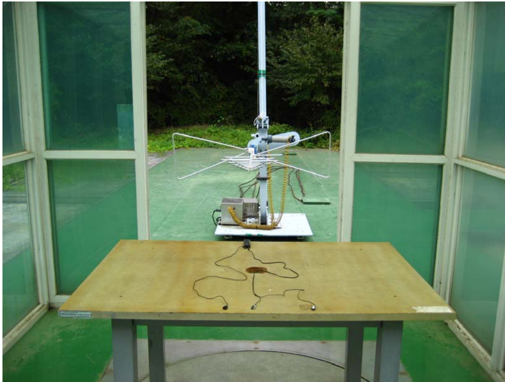
Radiated Emissions (Recording/Playback mode) Z-axis View
