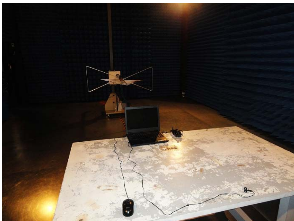
Radiated emission test view--
