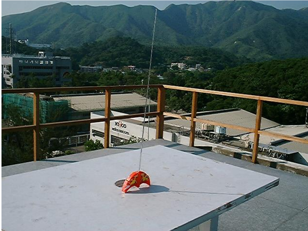
Measurement of Radiated Emission Test Set Up
