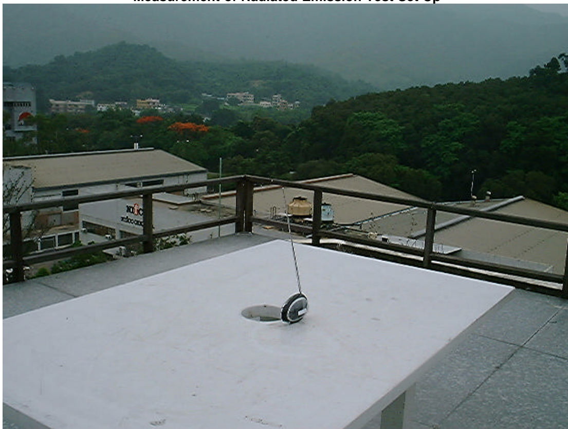
Measurement of Radiated Emission Test Set Up
