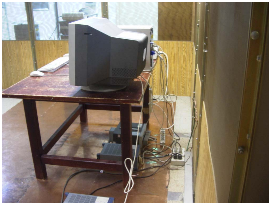
Conducted Emissions 150kHz - 30 MHz
