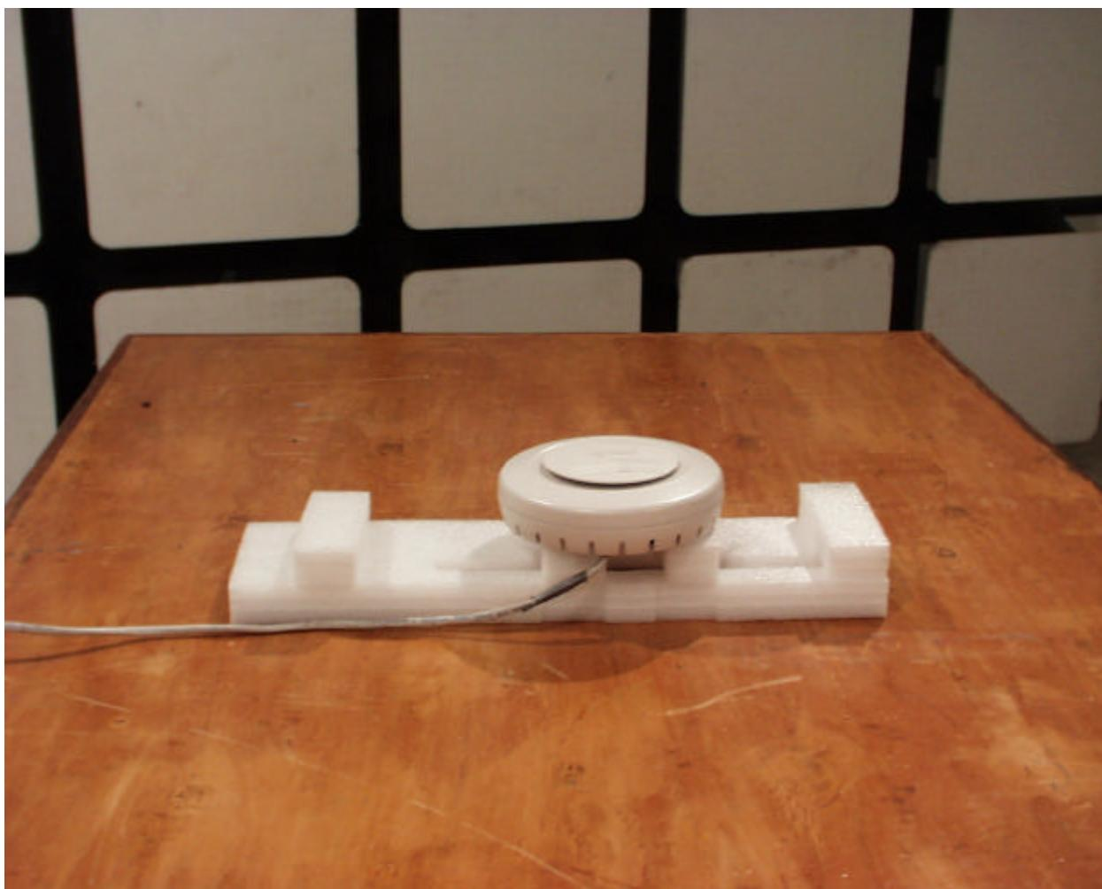
**DIGITAL DEVICE RADIATED EMISSIONS MEASUREMENT SETUP**
