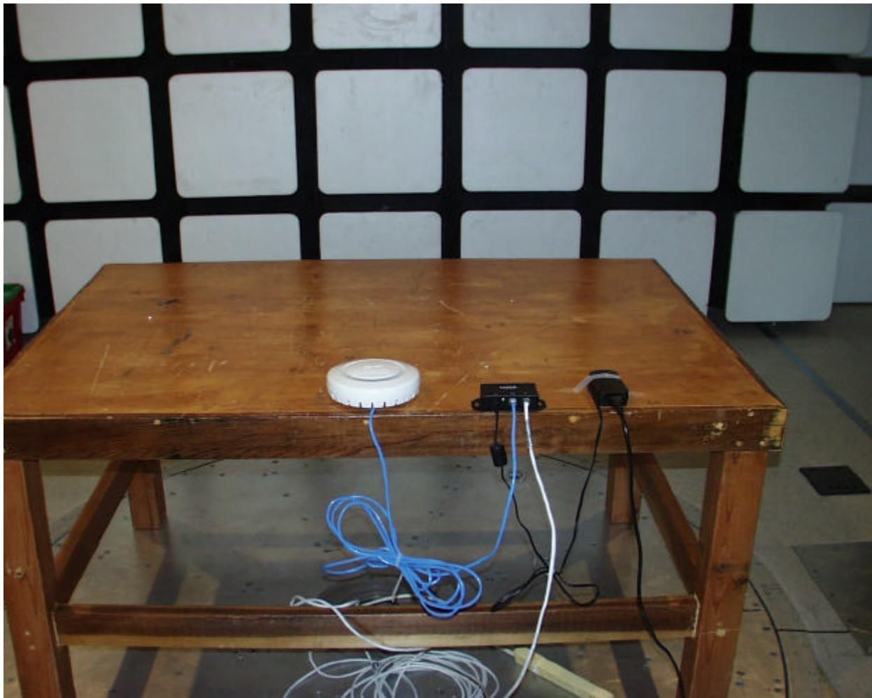
**POWERLINE CONDUCTED EMISSIONS MEASUREMENT SETUP**
