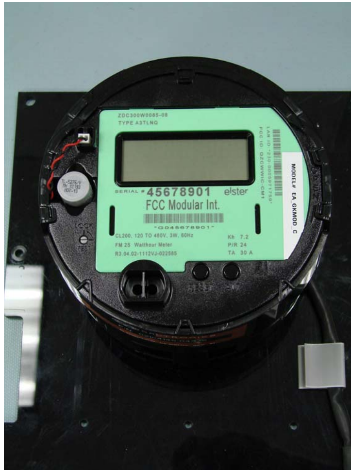
Modular EA_Gatekeeper with internal antennas completed assembly
