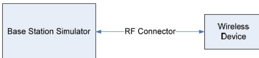
Figure 6-1. Conducted Power Test Setup Diagram
