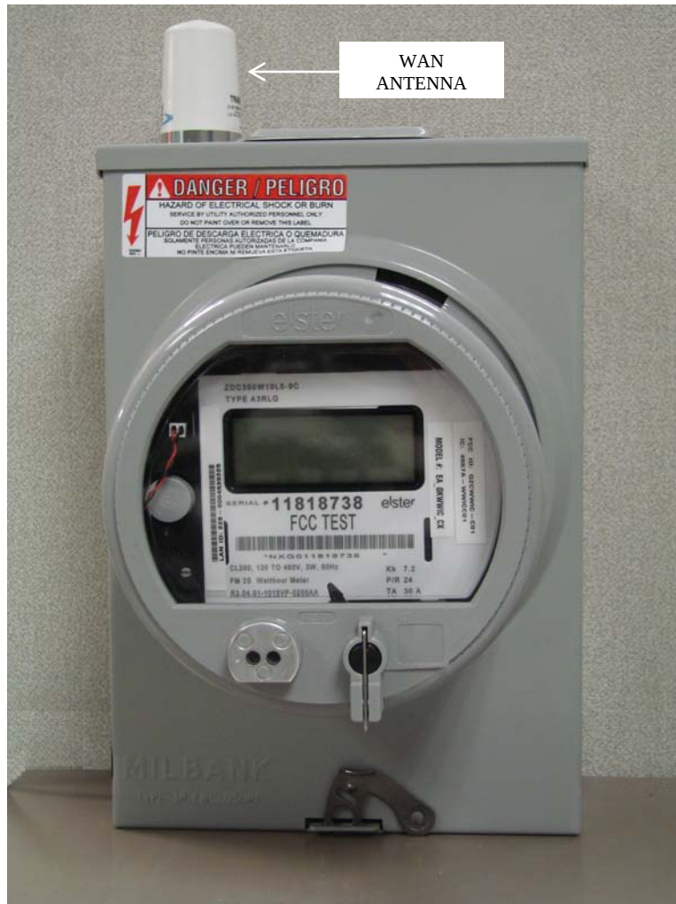
EA_Gatekeeper completed assembly
