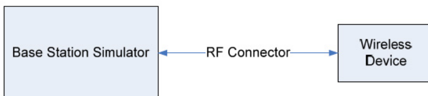
Figure 6-1. Conducted Power Test Setup Diagram
