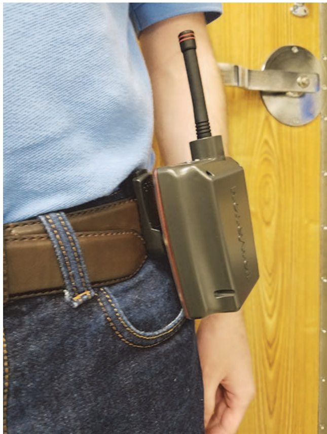
Figure 1. Correct position for wearing UFT with beltclip
