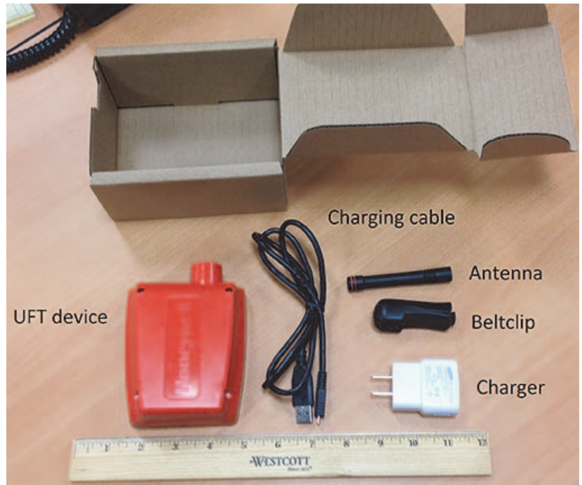
Figure 2. UFT with parts
