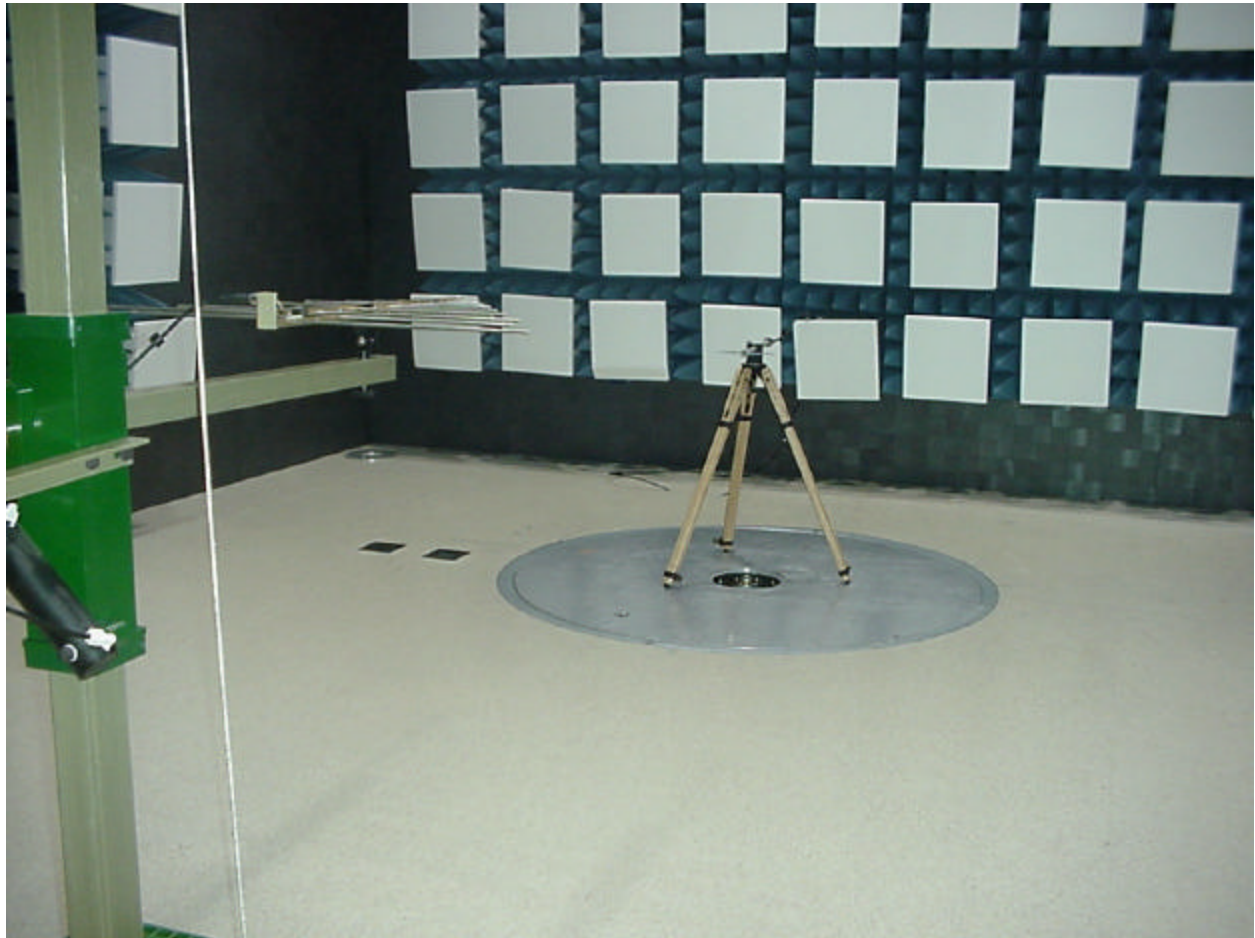
Figure 9 – Setup for Substitution Method
