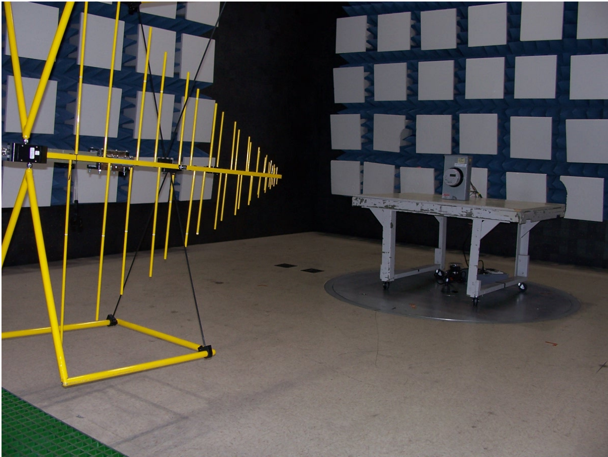
Radiated Emissions 30 MHz -1000 MHz Test Setup
