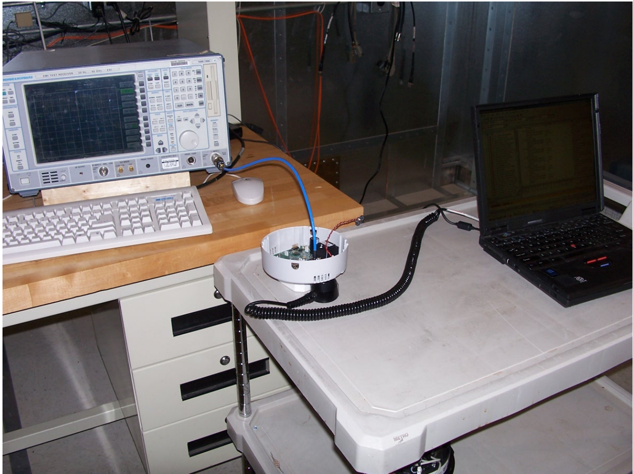
RF Conducted Emissions Test Setup
