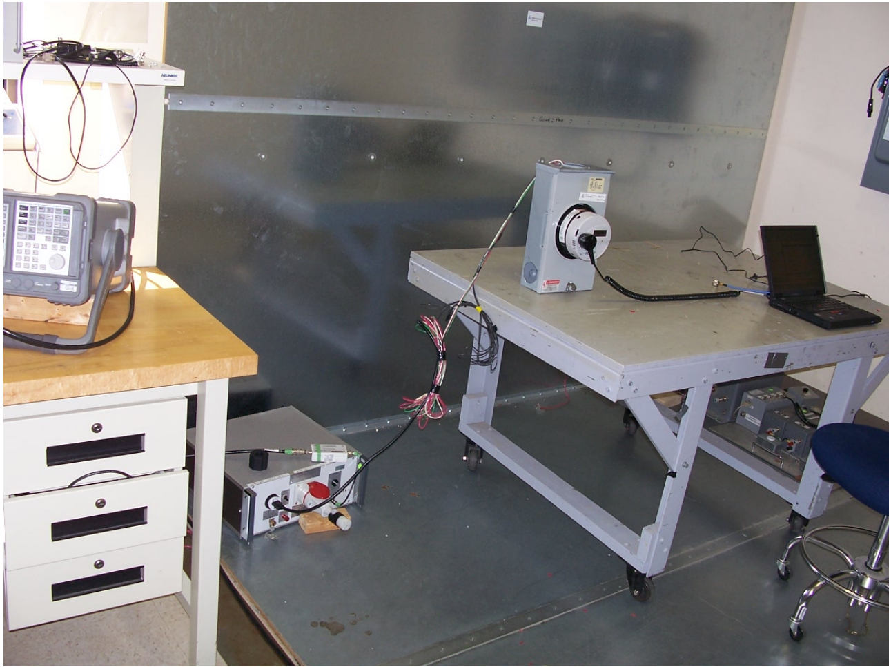
Power Line Conducted Emissions Test Setup
