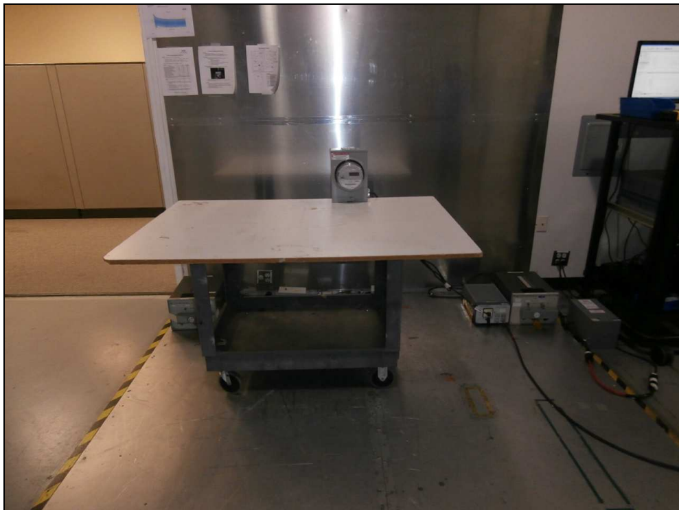
Figure 8: Conducted Emissions (Host)
