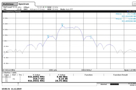
Figure 7.4.4.2-15: 20dB BW Mid Channel 150kbps
