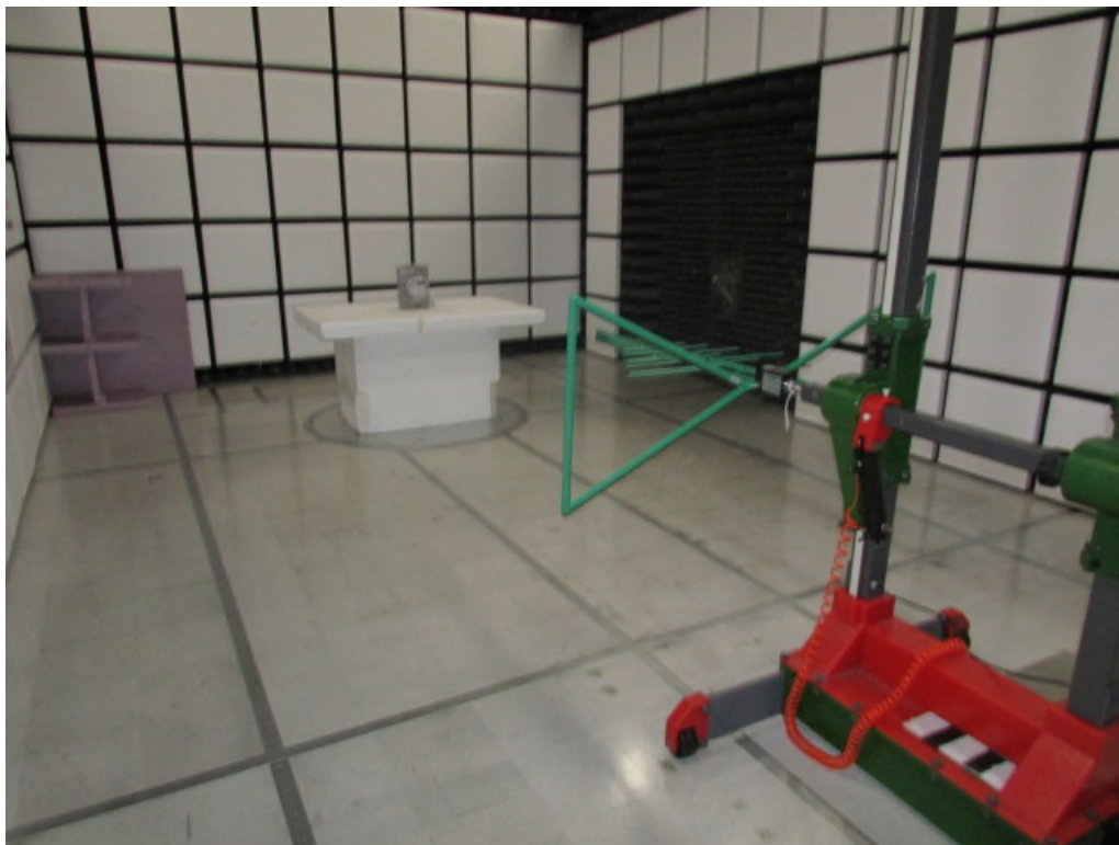
Figure 1: Radiated Emissions – Front – Below 1GHz
