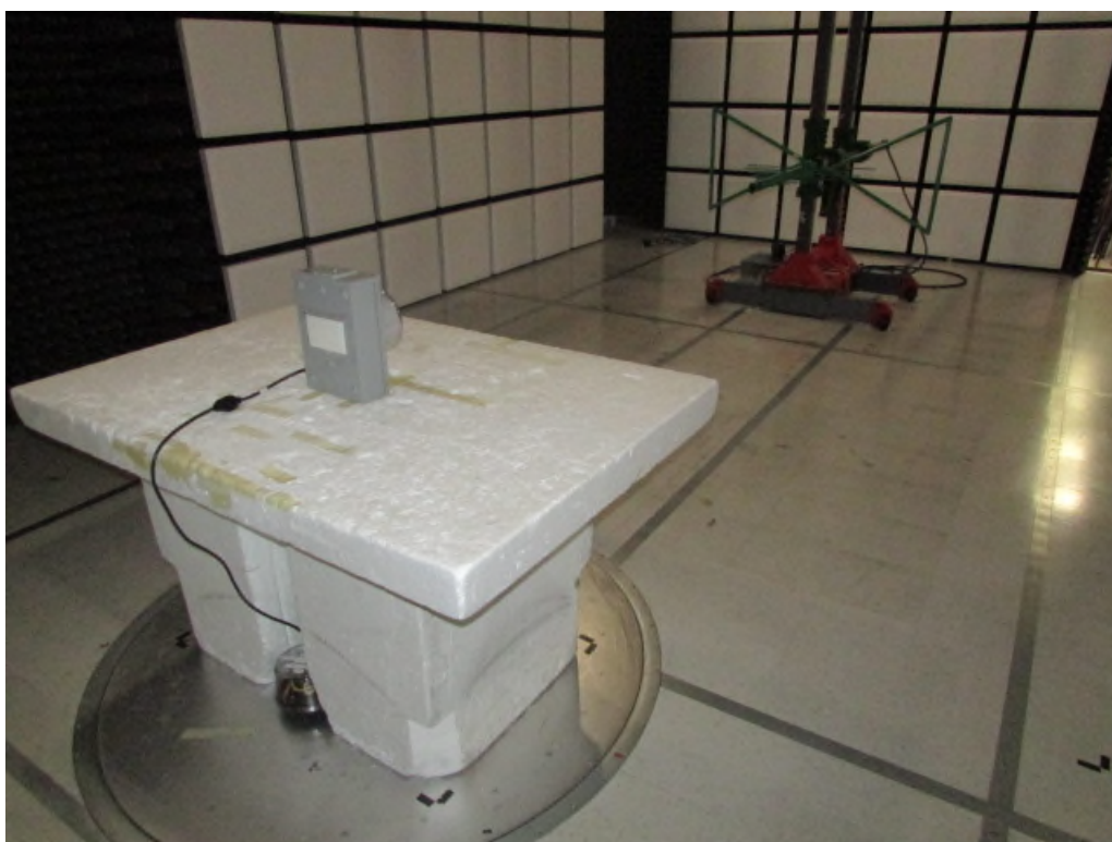
Figure 2: Radiated Emissions – Back – Below 1GHz
