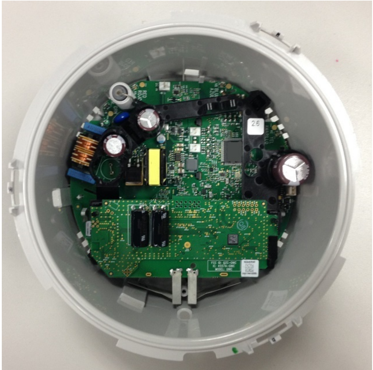
Figure 5: Module Installed in Sample Meter.
