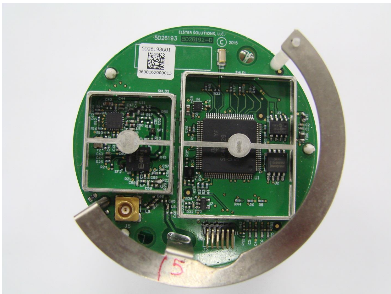
Radio PCBA, Top View, No Shields
