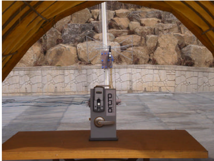
Photograph 1 : Setup for radiated Emissions
