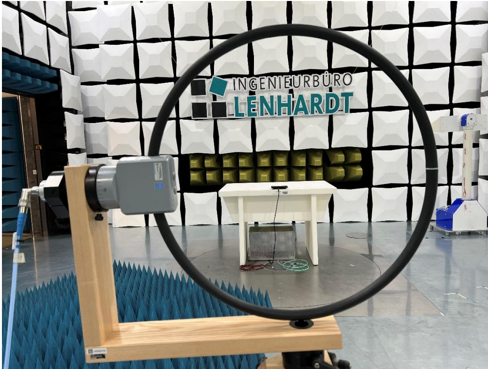
Photo No. 5, measurement in SAC, 9 kHz – 30 MHz, overall view:
