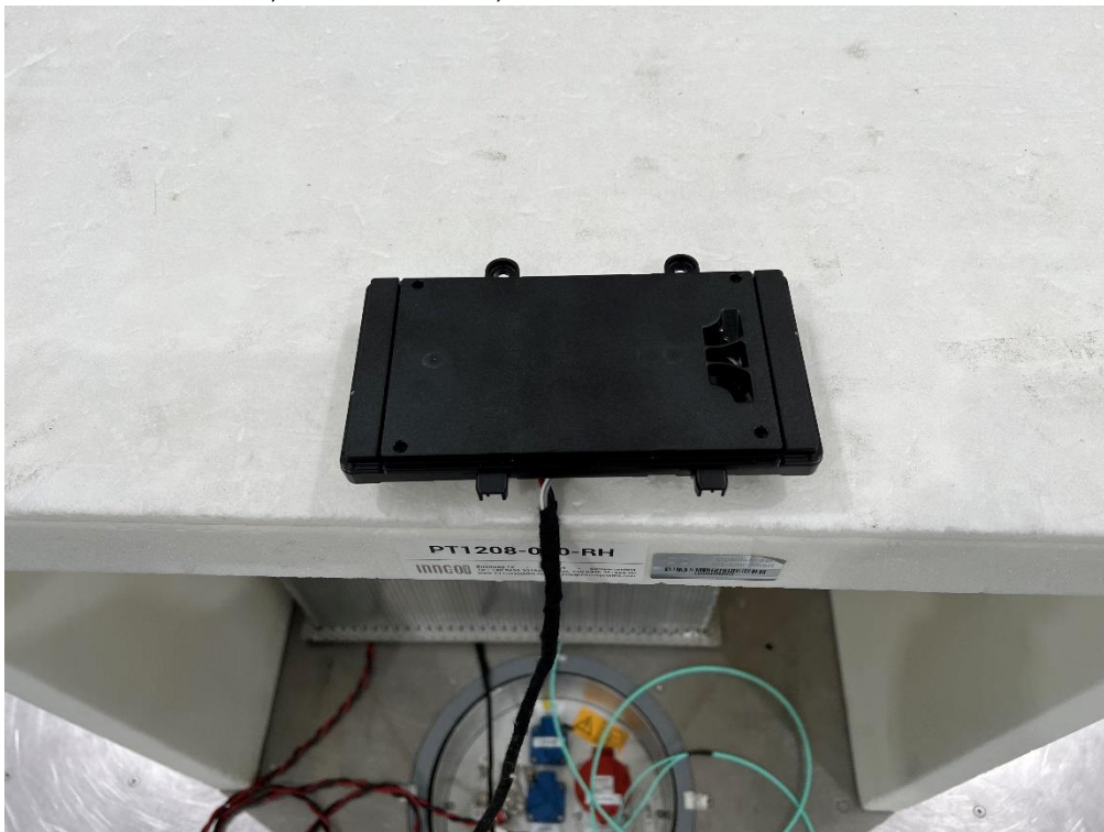
Photo No. 6, measurement in SAC, 9 kHz – 30 MHz, close view:
