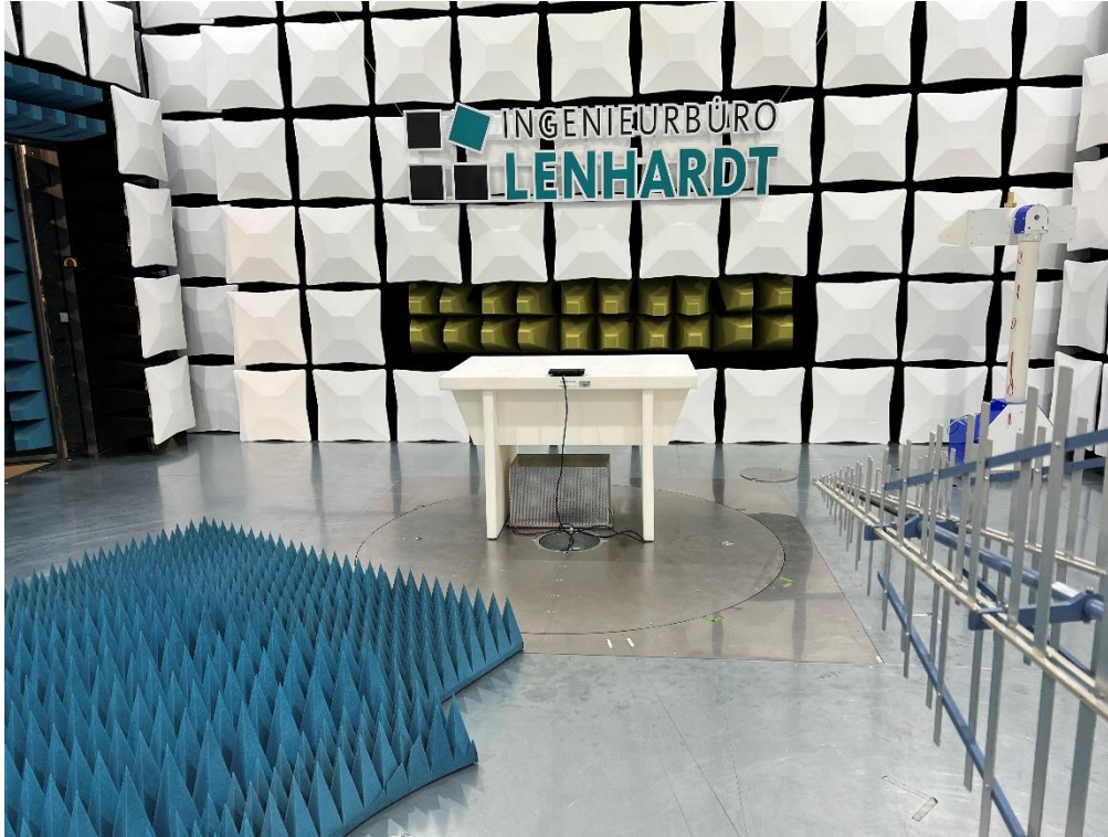
Photo No. 7, measurement in SAC, 30 MHz – 1 GHz, overall view:
