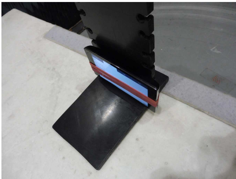
Photo 8: RSE set-up (30MHz to 1GHz)
