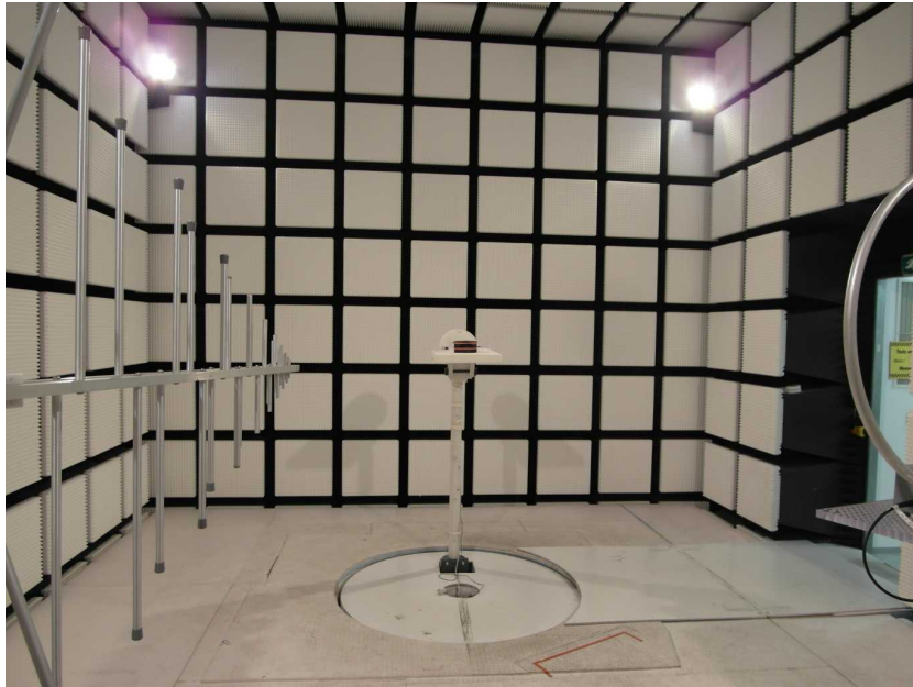
Photo 5: RSE set-up (>1GHz)
