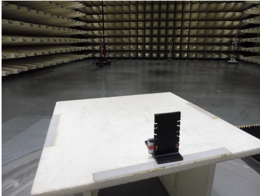
Photo 7: RSE set-up (30MHz to 1GHz)
