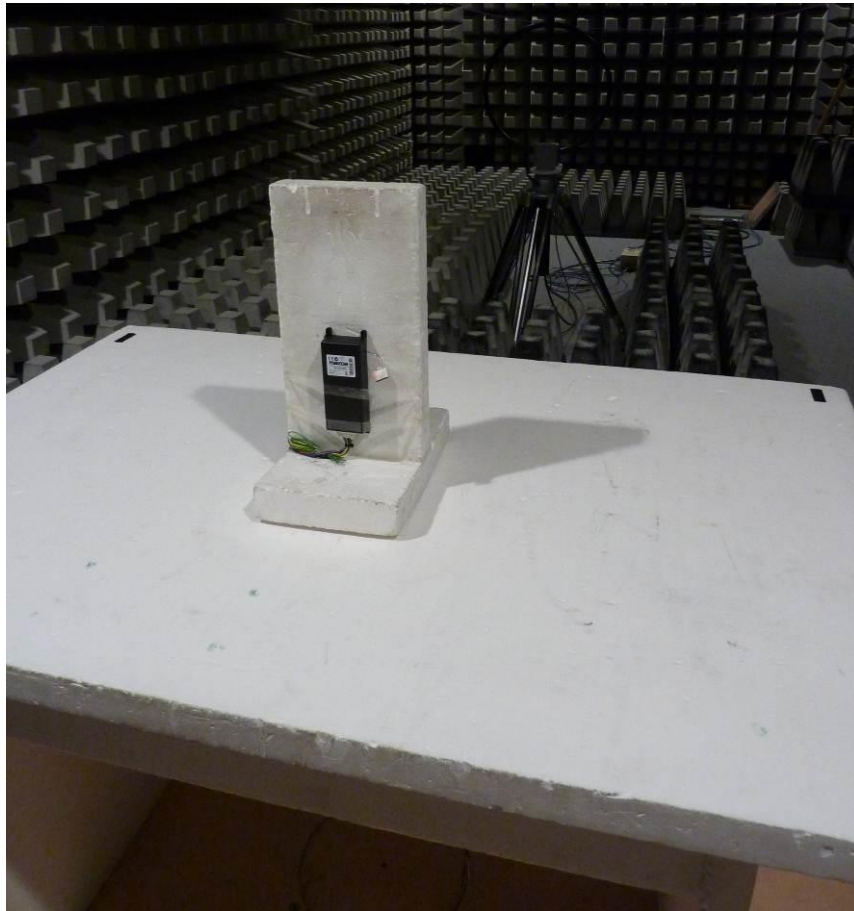
136031_15: Test setup - Radiated emission (fully anechoic chamber)
