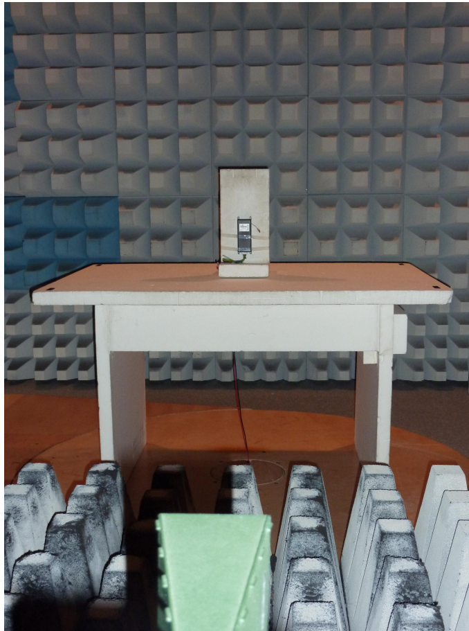
136031_18: Test setup - Radiated emission (fully anechoic chamber)
