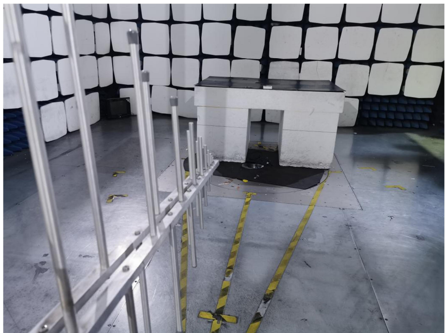
Radiation Emission Test Setup (30MHz to 1GHz)
