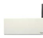
**NC551 Repeater:** Receives messages from system wireless devices and communicates them to the NC555 Gateway. The repeater receives system device messages on a 900MHz radio link and then relays each message to the gateway via 2.4GHz radio signals. The repeater is powered by an included PK505 Plug-in Transformer and a BA550 Backup Battery is included inside the repeater's housing.
