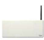
**NC555 Gateway:** Communicates messages from NC551 Repeaters to the Tek-BRIDGE™. The gateway receives signals from repeaters via 2.4GHz radio signals and relays information to the Tek-BRIDGE™ via TCP/IP Ethernet. The gateway is powered by an included PK505 Plug-in Transformer and a BA550 Backup Battery is included inside the gateway's housing.
