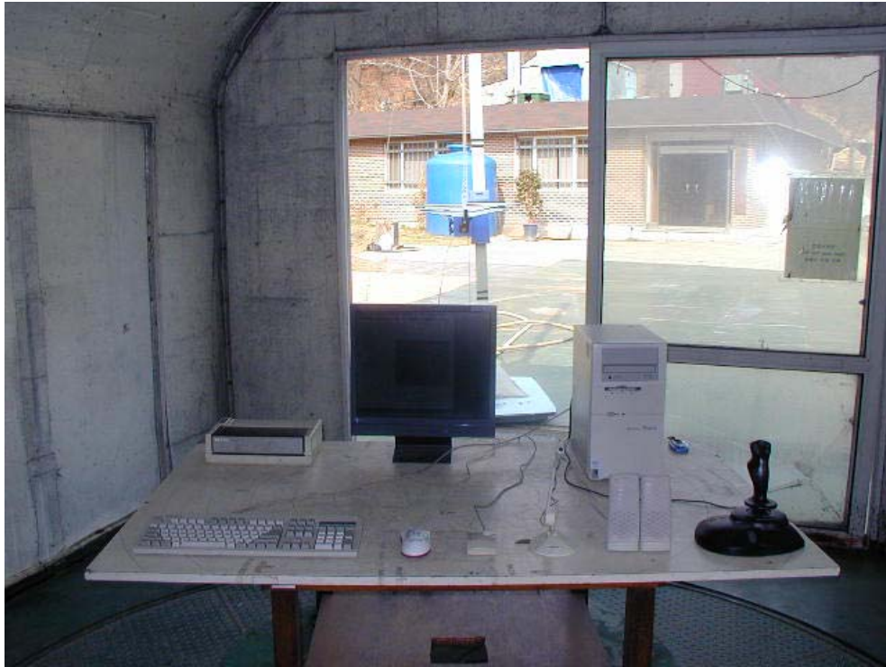
RADIATED EMISSION SETUP PHOTOGRAPH - FRONT VIEW ( 300- 1000 MHz )
