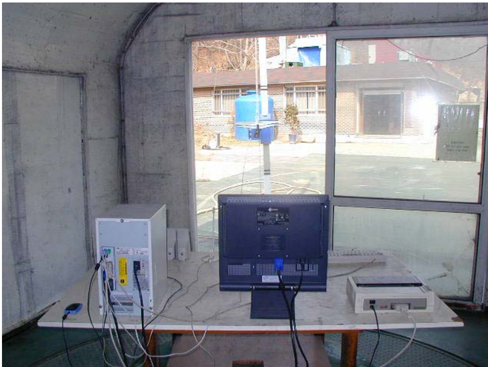
RADIATED EMISSION SETUP PHOTOGRAPH - REAR VIEW ( 300 - 1000 MHz )
