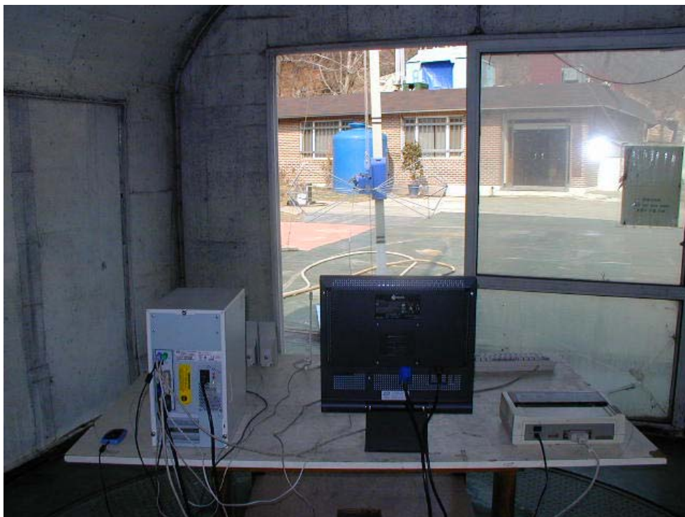
RADIATED EMISSION SETUP PHOTOGRAPH - REAR VIEW ( 30 - 300 MHz )
