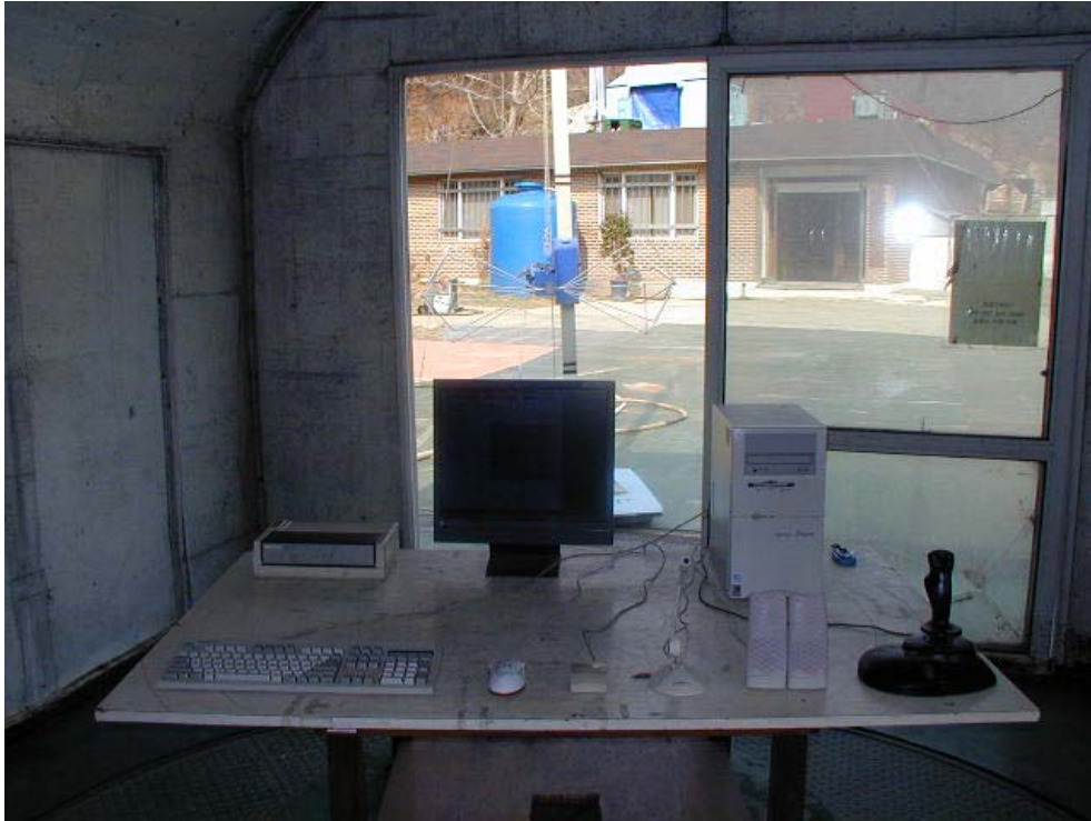
RADIATED EMISSION SETUP PHOTOGRAPH - FRONT VIEW ( 30 - 300 MHz )
