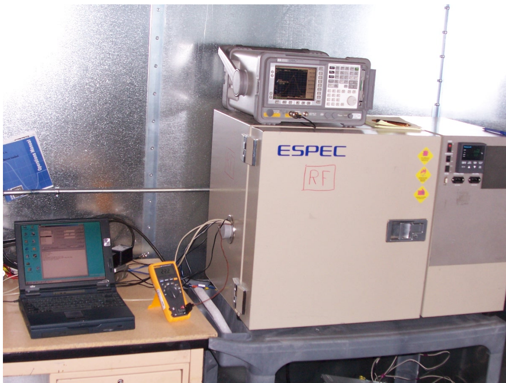
Figure 8 – Extreme Temperature test setup
