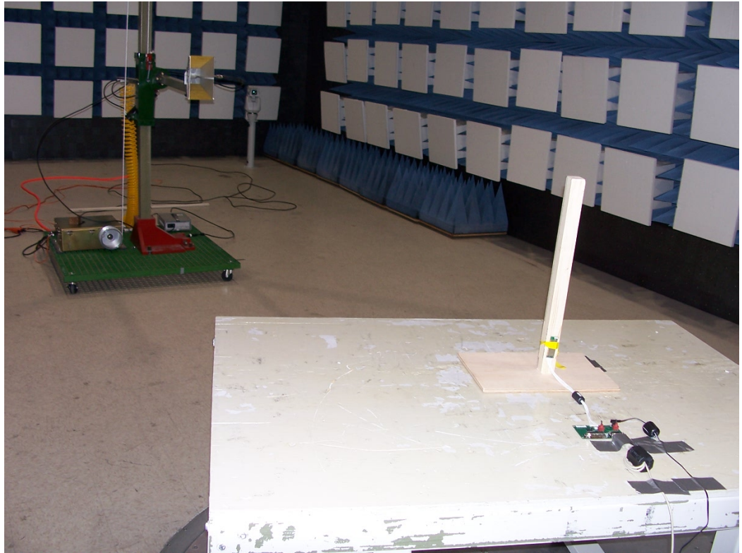
Figure 3 – Radiated emissions test setup (1GHz – 18GHz)
