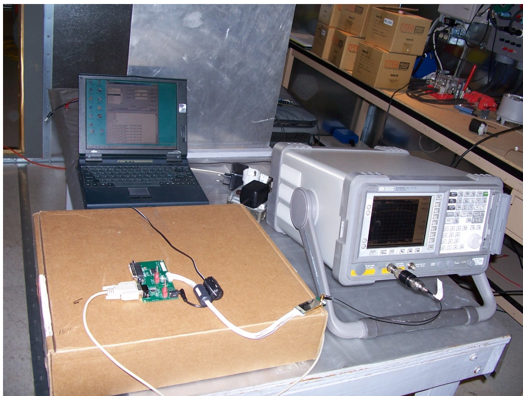
Figure 7 – Typical Conducted RF measurements using spectrum analyzer
