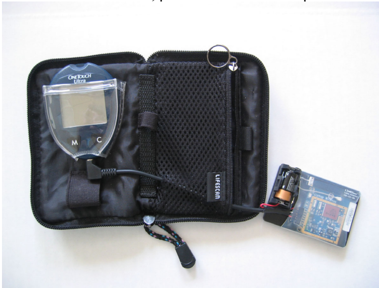
Figure 1: positioning of PWR-07-03 device. Please note that cable must pass through mesh, which may need to have a 1/4" cut made in it near the bottom left corner.
