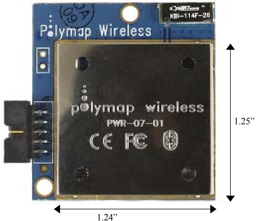
Label (see below) is stamped into the shield. Shield is soldered to the circuit board.
