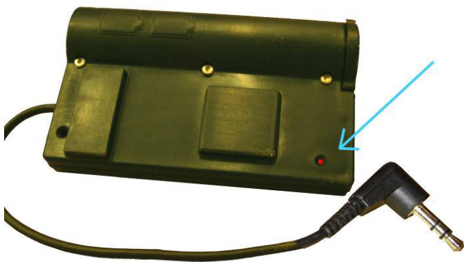
Figure 3: Please note the small indicator light located near the bottom right corner of the back side of the device. This allows the user to confirm whether the device is operating correctly
