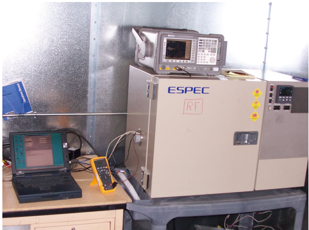
Figure 10 – Extreme Temperature test setup
