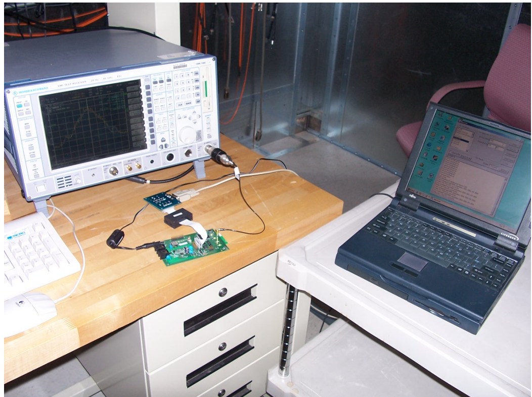
Figure 9 – Typical Conducted RF measurements using EMC receiver
