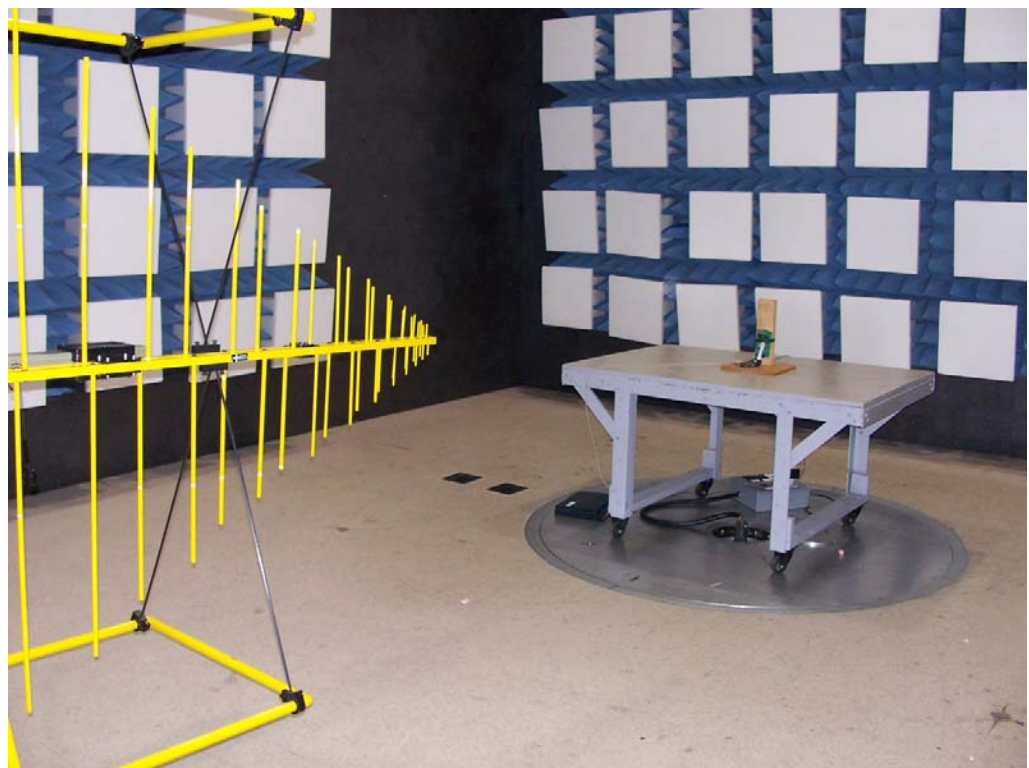
Figure 2 – Radiated emissions test setup (30MHz – 1GHz)
