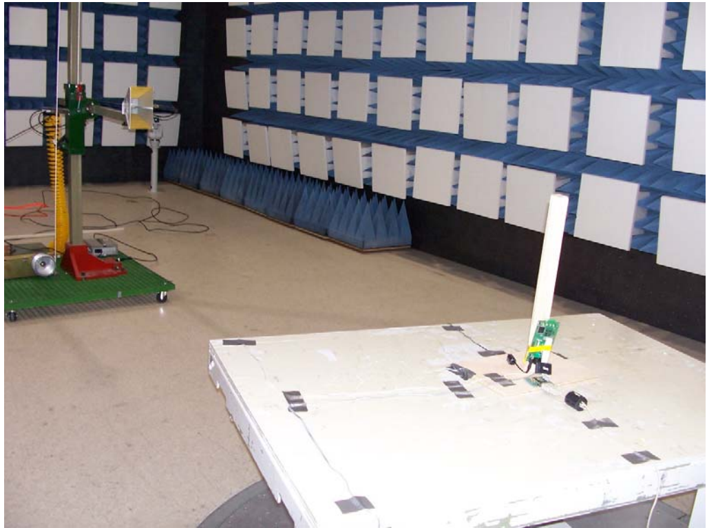
Figure 3 – Radiated emissions test setup (1GHz – 18GHz)
