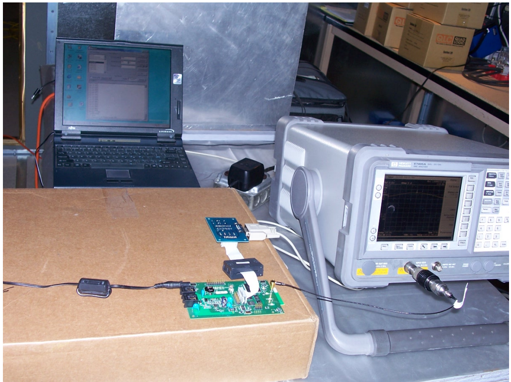
Figure 8 – Typical Conducted RF measurements using spectrum analyzer
