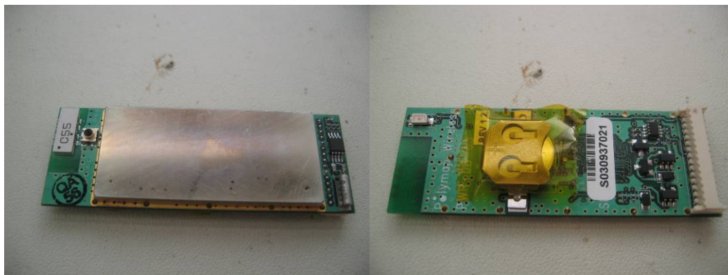
PWR-08-03, top and bottom views. Connector is at right edge of board. Battery provides a backup for a real-time clock.
