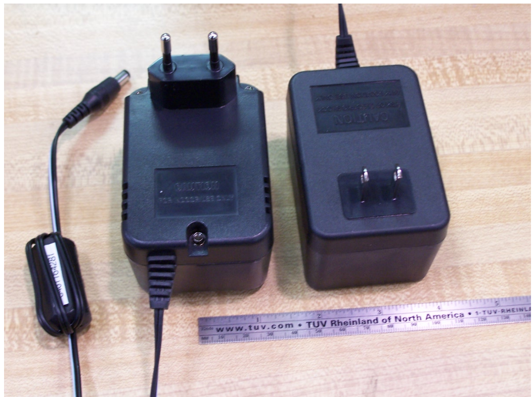
Figure 2 – View of power modules – 230V/50Hz, and 120V/60Hz shown
