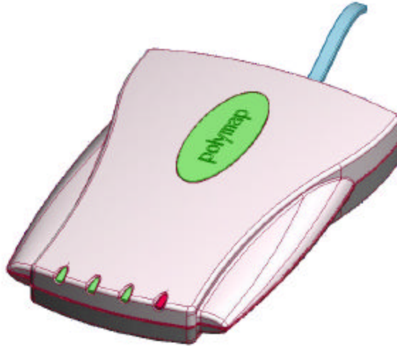
Figure 1: Access point, showing the four indicator lights: POWER, RADIO, TELEPHONE, and ERROR.
