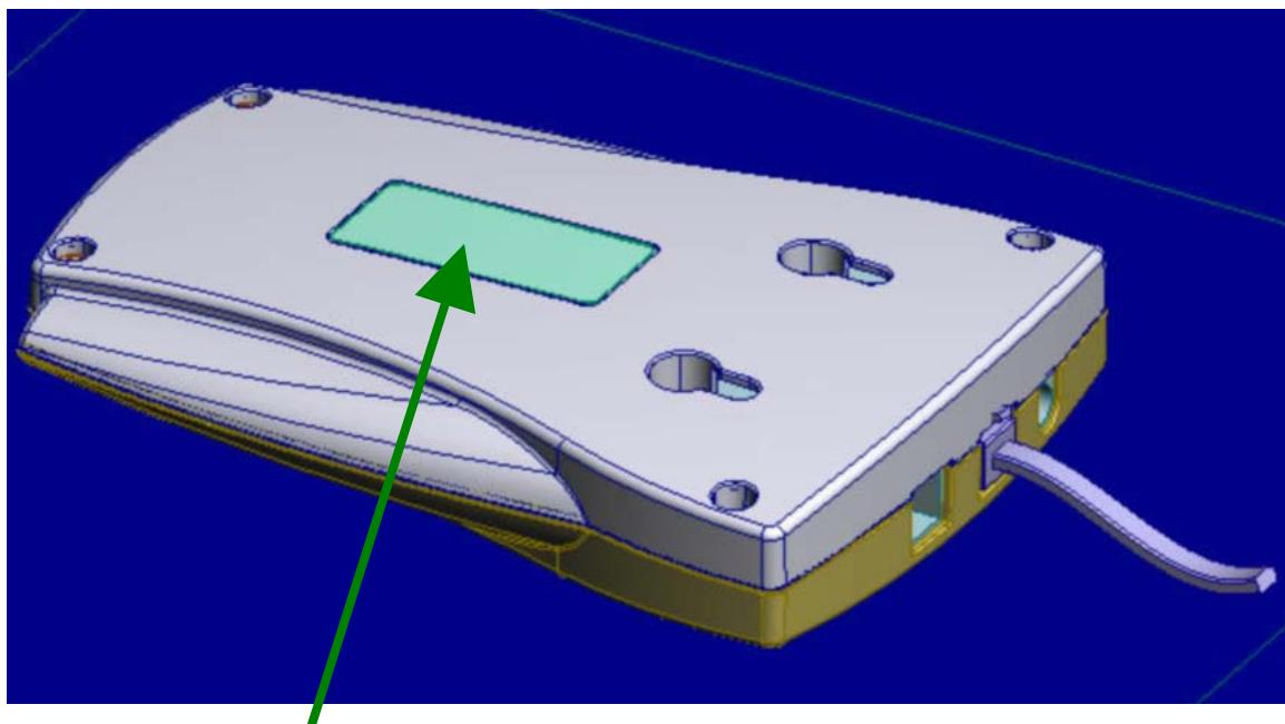
Label (see below) is located here on the bottom side of Base-Station/Access Point. It is made from a white polyester with lamination with a heavy-duty pressure sensitive adhesive to provide a permanent labeling solution.
