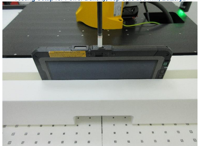
Testing Setup for Power Density, Top Side at 0 mm, Battery2
