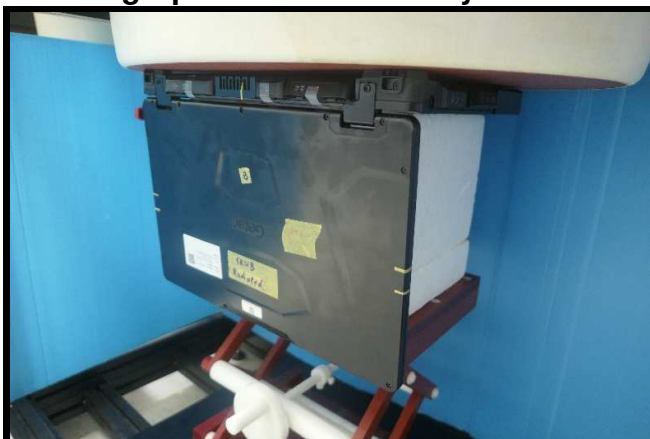
Bottom of Laptop Mode Tested at 0 mm
