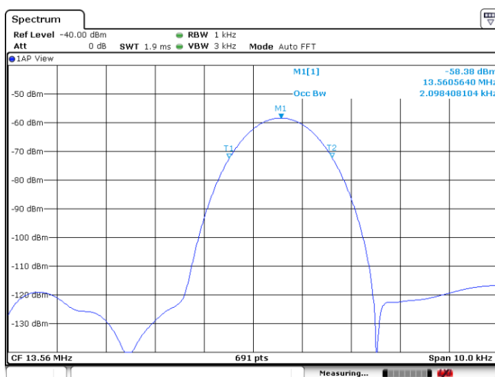
Emission Bandwidth Plot - 99% Bandwidth
